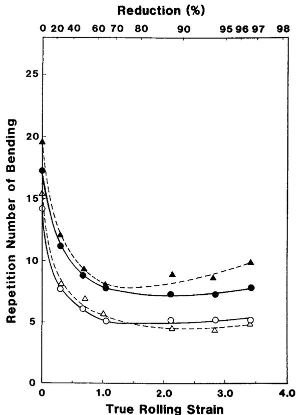
Figure 5 Repetition number of bending as a function of cold-rolling strain (see Fig. 3 caption). Alloy: Cu-0.26 wt% Cr-0.10 wt% Sn.
