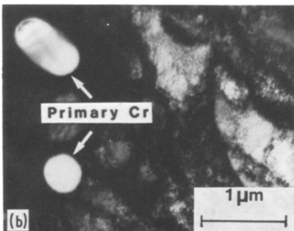
Figure 14 Transmission electron micrographs of Cu-0.81 wt % Cr-0.14 wt % Sn alloy. (a) Solution treatment + ageing,  $\epsilon = 0$ . (b) 25% roll + ageing,  $\epsilon = 0.288$ . (c) 67% roll + ageing,  $\epsilon = 1.109$ .  $\epsilon = \ln (h_0/h)$ .
