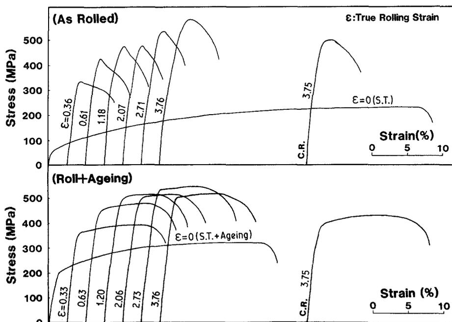
Figure 7 Stress-strain curves of Cu-0.81 wt % Cr-0.14 wt % Sn alloy. Specimens are rolled in the vertical direction. S.T., as solution treated; aged at 723 K for  $1.7 \times 10^3$  sec;  $\epsilon = \ln(h_0/h)$ ; C.R., cross rolling.
