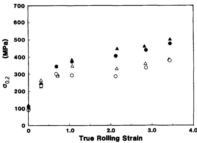
Figure 13 Relation between yield stress (0.2% offset) and rolling strain on Cu-0.26 wt %-0.10 wt % Sn alloy. For key, see Fig. 8 caption.
