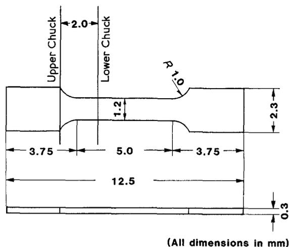
Figure 1 Shape and dimensions of repetition bending test and tensile test specimens.
