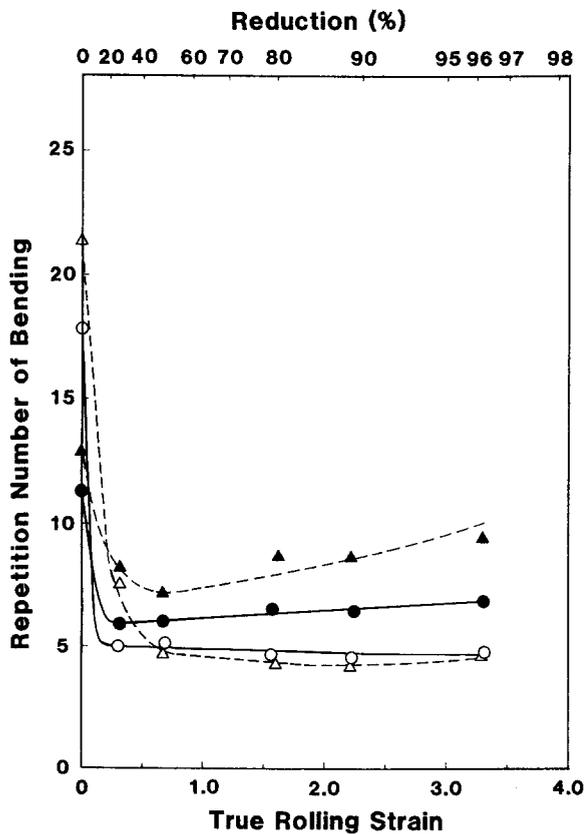
Figure 3 Repetition number of bending as a function of cold rolling strain  $\epsilon = \ln(h_0/h)$ , where  $h_0$  initial plate thickness,  $h$  plate thickness after cold rolling. Reduction  $[(h_0 - h)/h] \times 100$ ; solution treated (1223 K) before cold rolling; ageing at 723 K for  $1.8 \times 10^3$  sec; alloy, Cu-0.81 wt% Cr. Open symbols, roll only; solid symbols, roll and age. (O, ●) Parallel direction; ( $\Delta$ ,  $\blacktriangle$ ) vertical direction.
