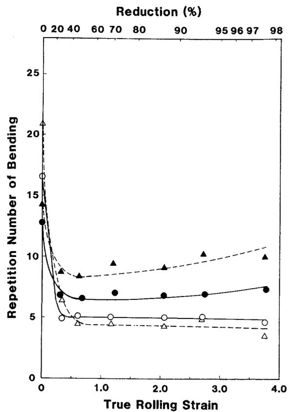
Figure 4 Repetition number of bending as a function of cold-rolling strain (see Fig. 3 caption). Alloy: Cu-0.81 wt% Cr-0.14 wt% Sn.
