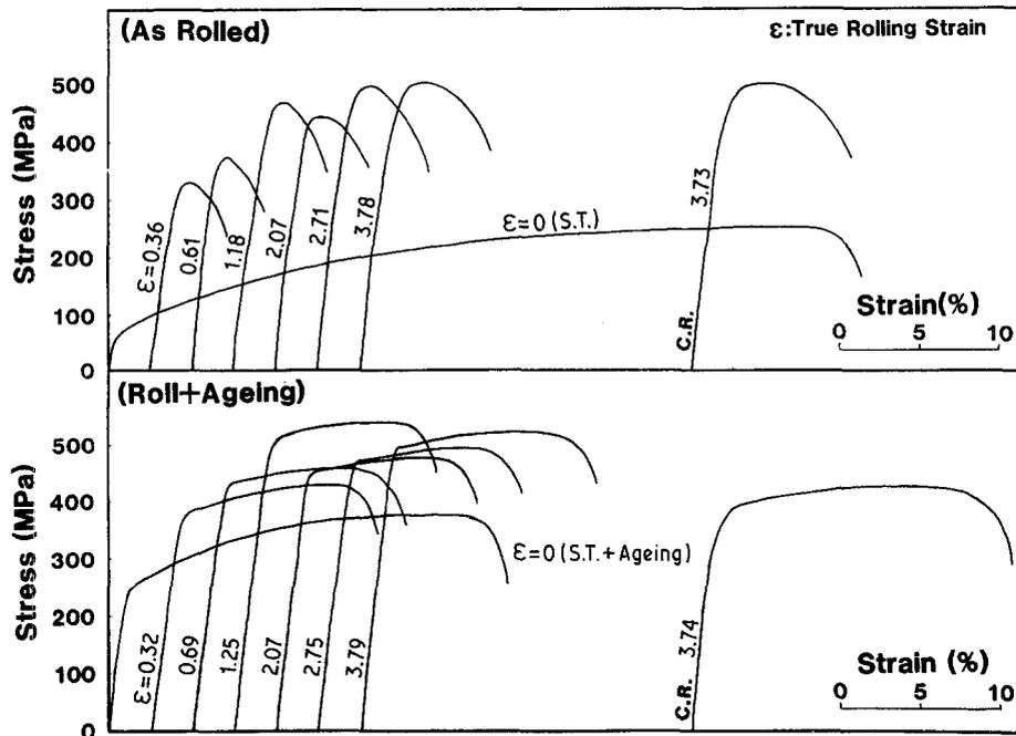
Figure 6 Stress-strain curves of Cu-0.81 wt % Cr-0.14 wt % Sn alloy. Specimens are rolled in the parallel direction. S.T., as solution treated; aged at 723 K for  $1.7 \times 10^3$  sec;  $\epsilon = \ln(h_0/h)$ ; C.R., cross rolling.
