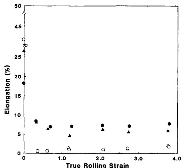
Figure 9 Relation between fracture elongation and rolling strain on Cu-0.81 wt % Cr-0.14 wt % Sn alloy cold rolled, and aged after cold rolling. For key, see Fig. 8 caption.
