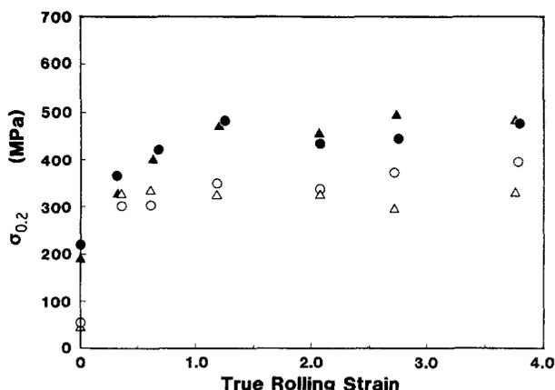
Figure 12 Relation between yield stress (0.2% offset) and rolling strain on Cu-0.81 wt % Cr-0.14 wt % Sn alloy. For key, see Fig. 8 caption.
