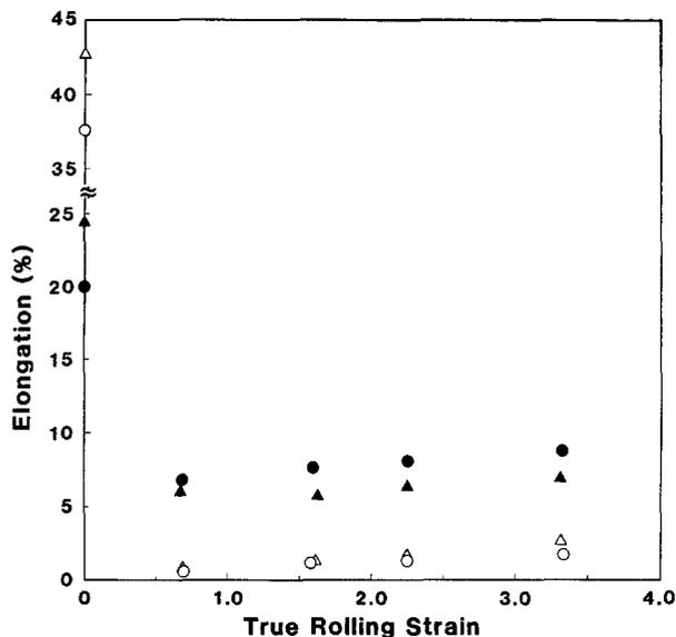
Figure 8 Relationship between fracture elongation and rolling strain on Cu-0.81 wt % Cr alloy cold rolled (open symbols), and aged after cold rolling (solid symbols). (O, ●) Parallel direction, (Δ, ▲) vertical direction.
