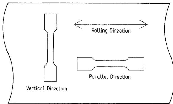
Figure 2 Relationship between rolling direction and longitudinal axis of specimen. Parallel direction: rolling direction is parallel to longitudinal axis of specimen. Vertical direction: rolling direction is vertical to longitudinal axis of specimen.
