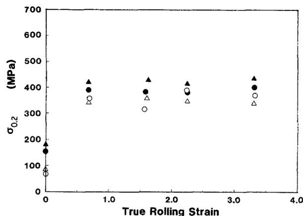
Figure 11 Relation between yield stress (0.2% offset) and rolling strain on Cu-0.81 wt % Cr alloy. For key, see Fig. 8 caption.
