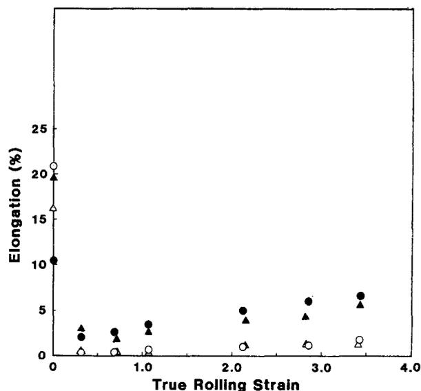
Figure 10 Relation between fracture elongation and rolling strain on Cu-0.26 wt % Cr-0.10 wt % Sn alloy cold rolled, and aged after cold rolling. For key, see Fig. 8 caption.
